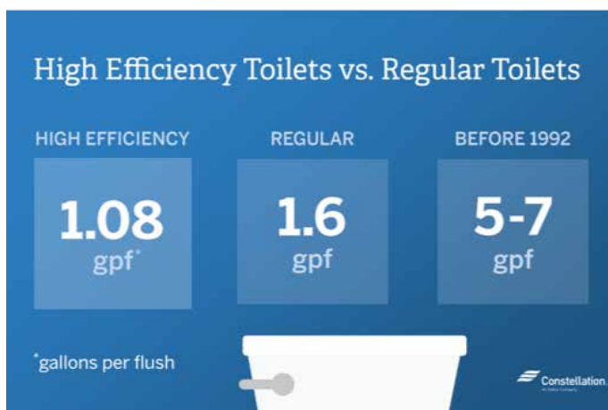
Figure 3: High Efficiency Toilets and Water Use. Retrieved from: https://www.dfcbelize.org/energy-efficiency-technologies/
